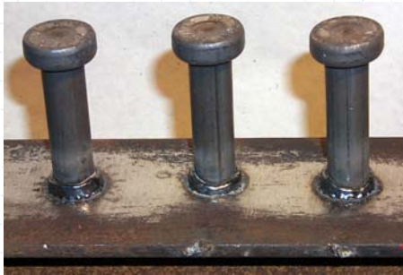
Studs welded to the steel beam
